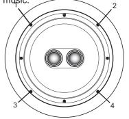
Tighten all four of the mounting screws in the same manner until the speaker is properly aligned and held tight to the wall surface. *Caution: Do not over tighten!*
